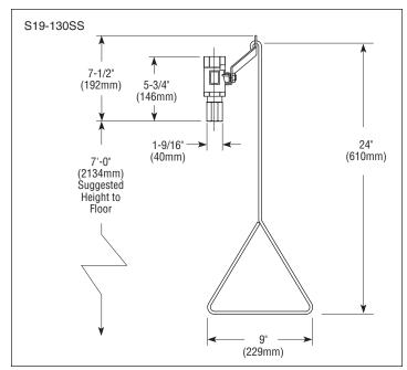
NOTE: All dimensions assume standard thread engagement. Variations in manufacturing allow for +/- 1/8" (3mm) per threaded joint. To find the tolerance of a dimension, add the number of thread joints in between a dimension and multiply it by 1/8" (3mm).
